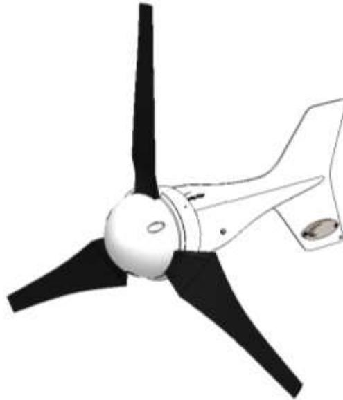
Fig-9: Attach the nose cone
