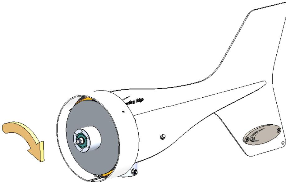
Fig-4: Checking magnet rotor rotation and coil-disc continuity
