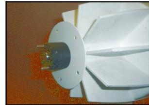
Offer rotor blade assembly up to rotor hub spacer and slide into place.
