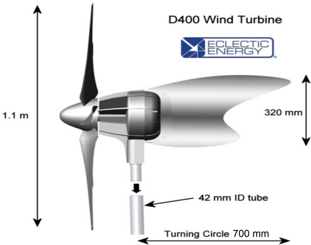
Rated outputs 225 watts at 11 m/s, 400 watts at 16.5 m/s
